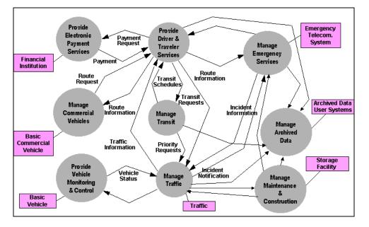
Figure 1. Simplified Top Level Logical Architecture
